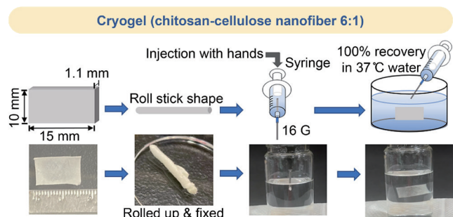
Fig. 5: Injected rod cryogel forms a large sheet of cryogel. [Reproduced from Ref. 3]
